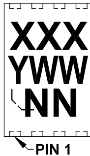
8-Lead TDFN (2x3x0.75 mm)
