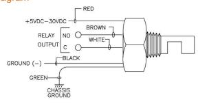
Figure 2 Typical wiring diagram for LL-01 series elements
