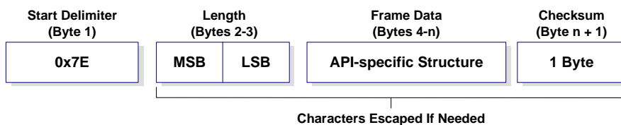
Figure 7-02. UART Data Frame Structure - with escape control characters:
