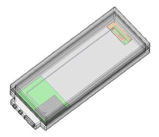
Position 2. Antenna could be mounted on upright position at bottom end of device
