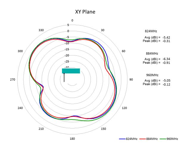
Note: Antenna tested on 2mm plastic plate with 200mm feed cable.
