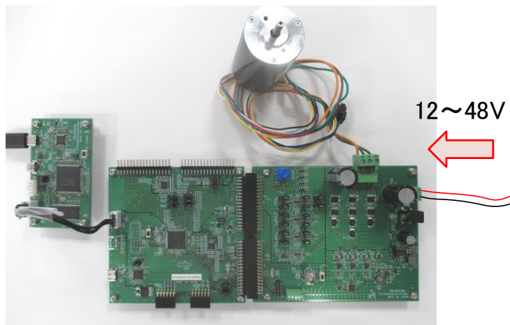
Figure 4-11 Power supply from terminal block
