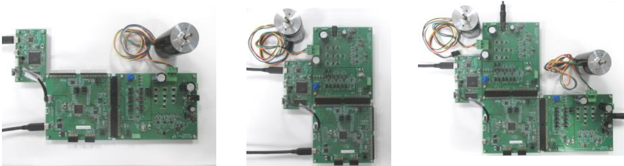
(1)CPU board + INV board (connected with CN1,CN2)
