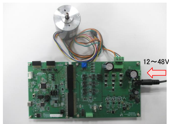
Figure 4-10 Power supply from DC jack
