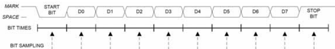
Figure 22.4. UART0 Mode 1 Timing Diagram
