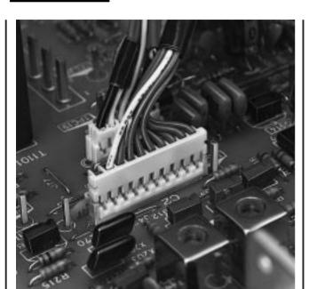
This 2.5mm (.098") pitch connector for printed circuit boards has an ultra-thin construction. It was developed by combining the technology of our best crimp style connectors, and the technology of our best insulation displacement connectors. The in-line method provides high-density capability to the end user.
