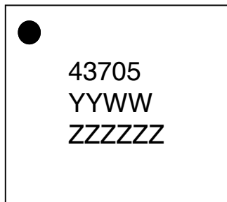
Figure 33. Top Marking Specification
