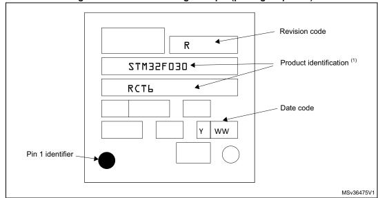
Figure 30. LQFP64 marking example (package top view)
