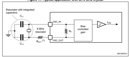
Figure 17. Typical application with an 8 MHz crystal
