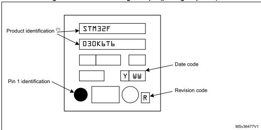
Figure 36. LQFP32 marking example (package top view)
