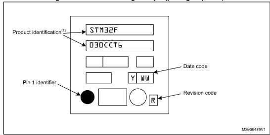
Figure 33. LQFP48 marking example (package top view)
