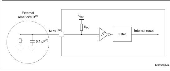
Figure 22. Recommended NRST pin protection
