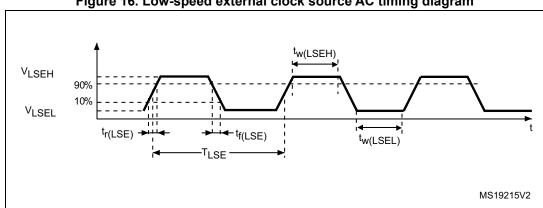
Figure 16. Low-speed external clock source AC timing diagram
