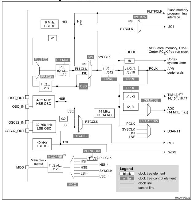
Figure 2. Clock tree of STM32F030x4/x6/x8
