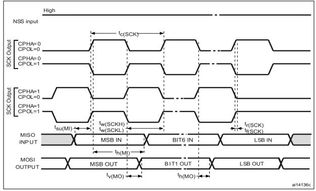
Figure 27. SPI timing diagram - master mode
