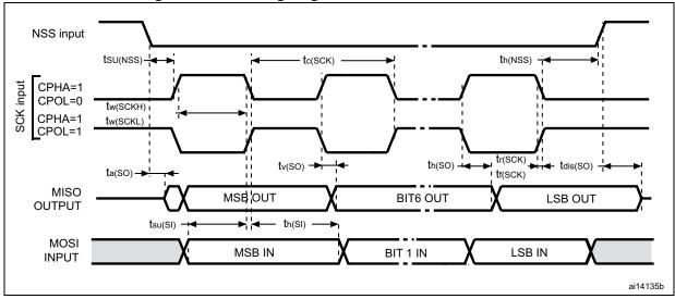
1. Measurement points are done at CMOS levels: 0.3  $\rm V_{DD}$  and 0.7  $\rm V_{DD}.$
