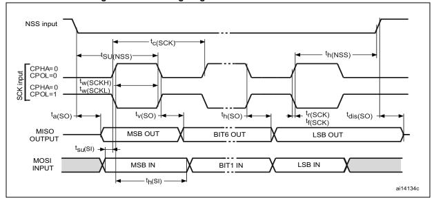
Figure 25. SPI timing diagram - slave mode and CPHA = 0
