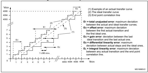
Figure 23. ADC accuracy characteristics
