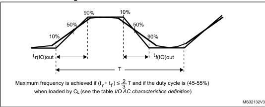
Figure 21. I/O AC characteristics definition
