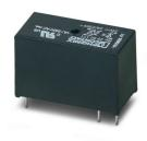
Plug-in miniature solid-state relay, power solid-state relay, 1 N/O contact, input: 24 V DC, output: 24 - 253 V AC/2 A
