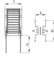
General InformationSeriesSCFStyleThrough-HoleRoHSYesNotesLead Spacing (S/S1) Are For Reference Only.MiscellaneousTemperature Rise Maximum: 60 K.CoreNanocrystal
