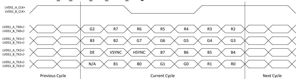
Figure 6: 24-bit / 18-bit Compatible Colour Mapping (Intel 24.0 LVDS Data Format)
