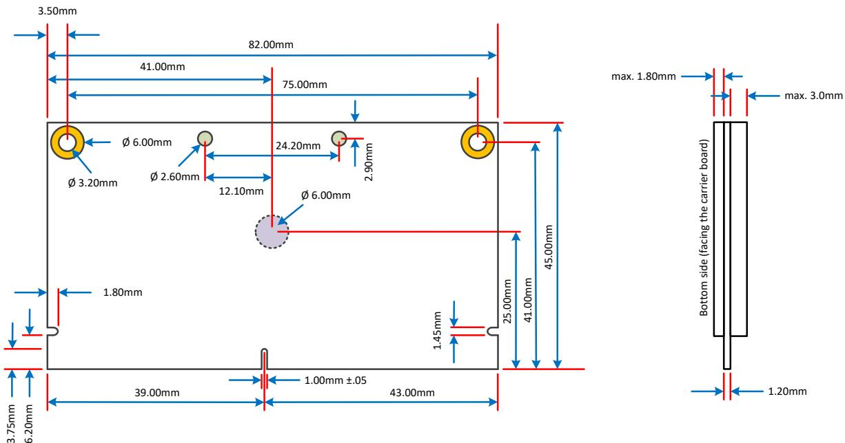
Figure 12 Mechanical dimensions of the Apalis module (top view)
