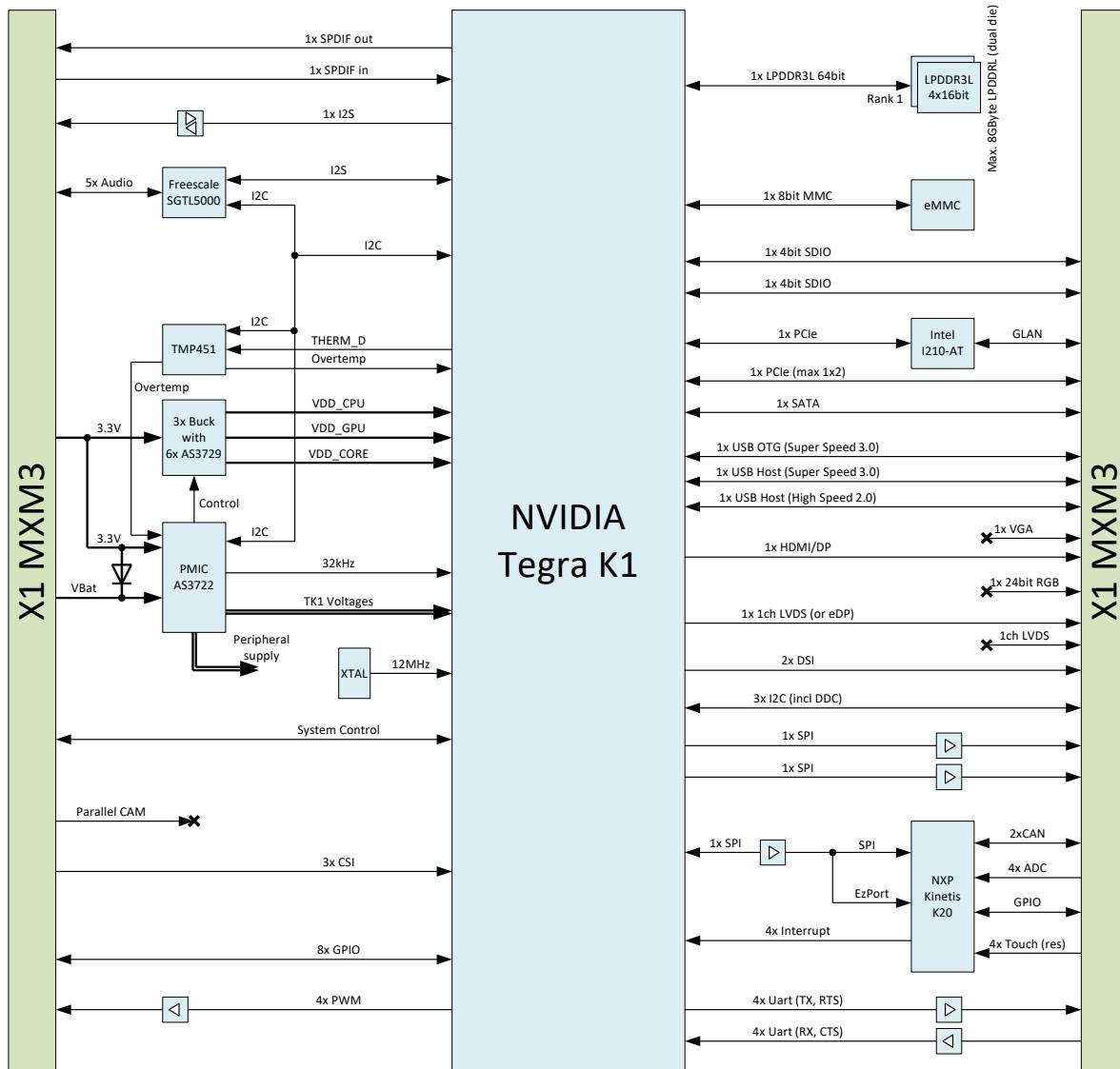
Figure 2 Apalis TK1 Block Diagram
