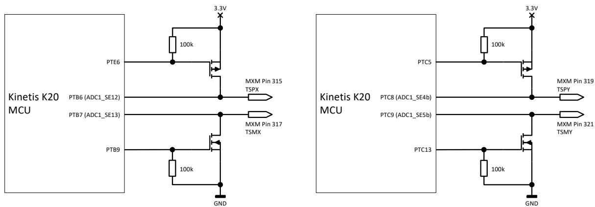
Figure 9: External Circuit for Touch Panel Interface
