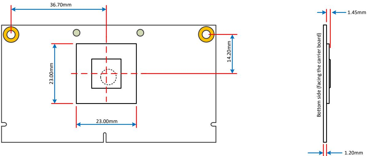
Figure 13 Mechanical position of NVIDIA Tegra K1 SoC (top view)
