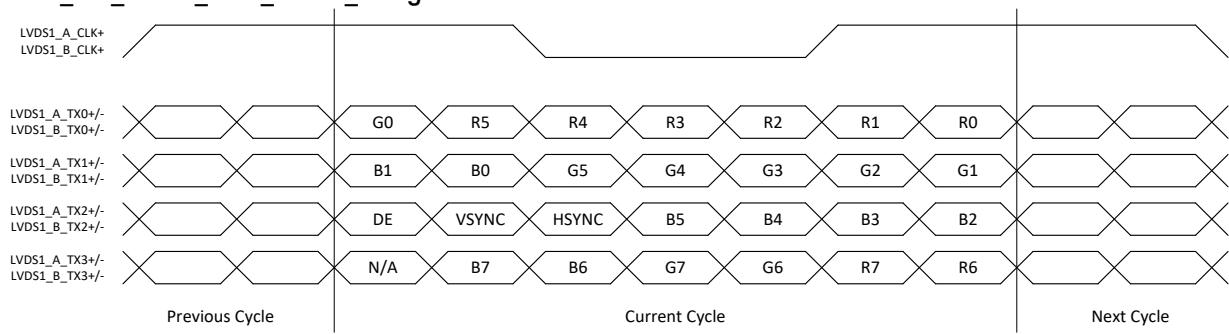
Figure 7: Common 24-bit VESA Colour Mapping (Intel 24.1 LVDS Data Format)
