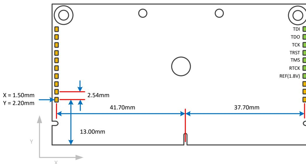
Figure 10 JTAG test point location on bottom side of module
