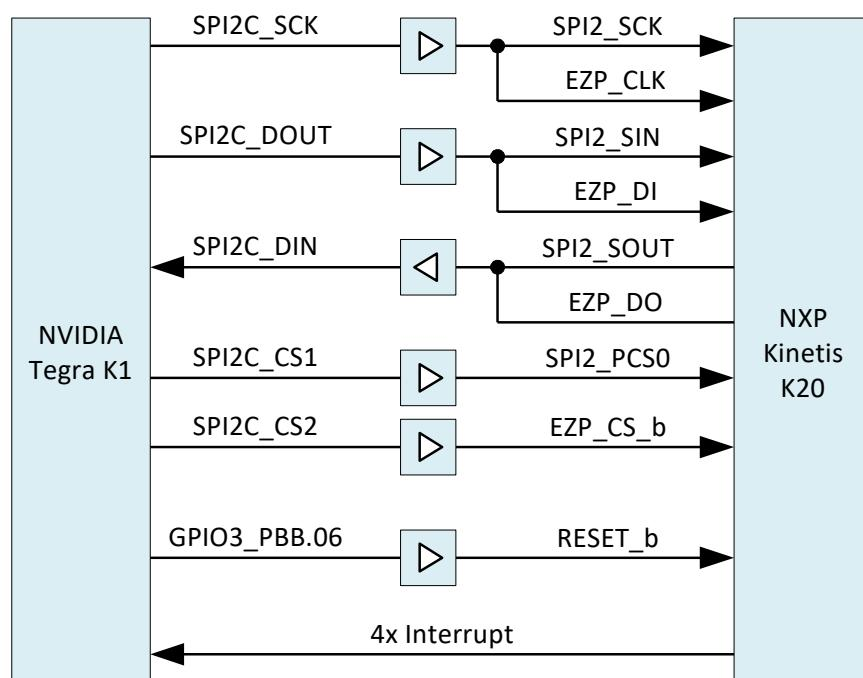
Figure 5: Connections between SoC and MCU
