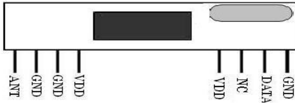
Figure1 CY02 Shape & Pins
