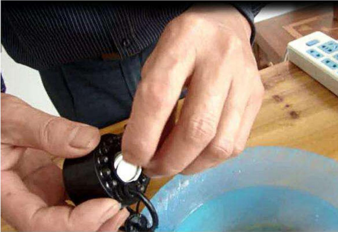
3) change the new piezoceramics. turn the black part clockwise to tighten the bit as picture.
