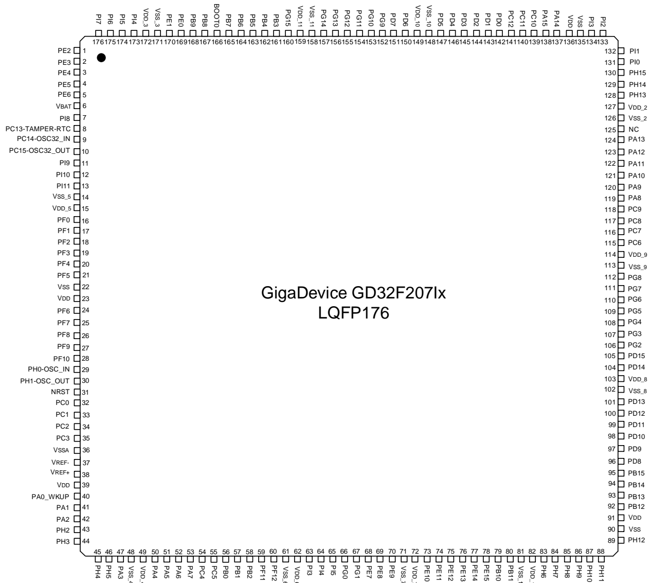
Figure 2. GD32F207Ix LQFP176 pinouts
