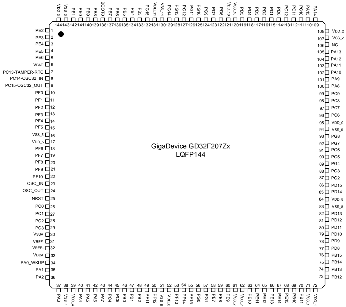
Figure 3. GD32F207Zx LQFP144 pinouts
