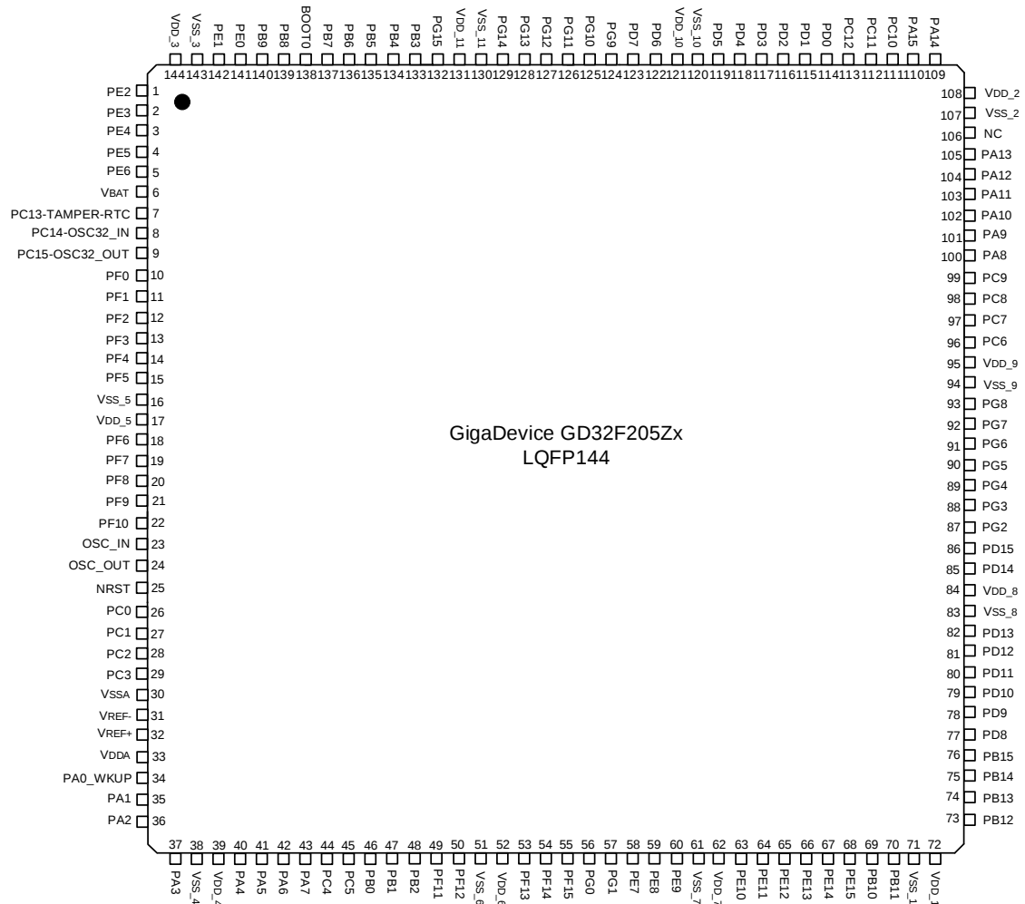
Figure 2. GD32F205Zx LQFP144 pinouts
