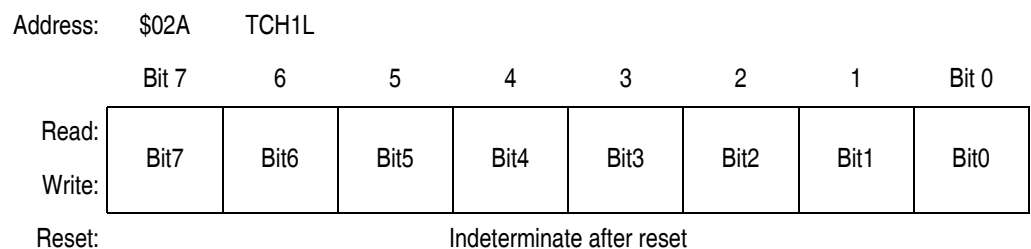
Figure 10-9. TIM Channel Registers (TCH0H/L:TCH1H/L)
