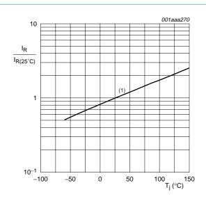
(1) PESD3V3S1UB;  $V_{RWM}$  = 3.3 V PESD5V0S1UB;  $V_{RWM}$  = 5 V  $I_{R}$  is less than 10 nA at 150 °C for: PESD12VS1UB;  $V_{RWM}$  = 12 V PESD15VS1UB;  $V_{RWM}$  = 15 V PESD24VS1UB;  $V_{RWM}$  = 24 V
