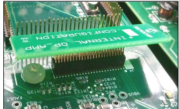
FIGURE 1: INTERNAL OP AMP CONFIGURATION BOARD
