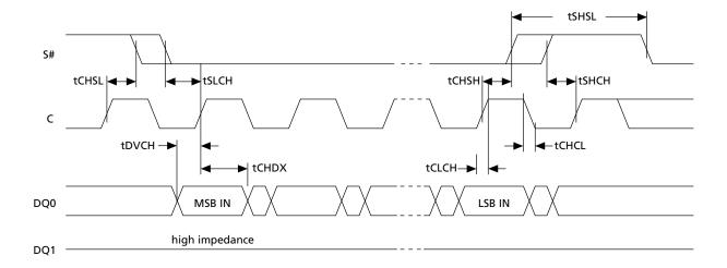
Figure 24: Write Protect Setup and Hold during WRSR when SRWD=1 Timing
