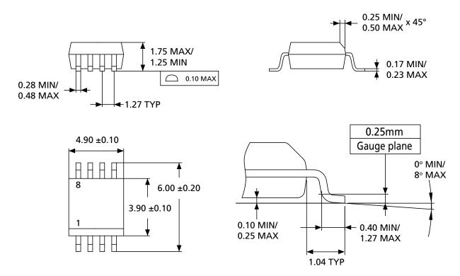
Notes: 1. The 1 that appears in the top view of the package indicates the position of pin 1.
