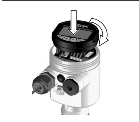
Fig. 26: Installation of the indicating and adjustment module
