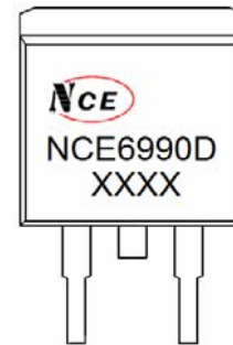
Marking and pin assignment
