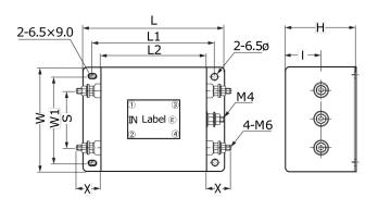
**General Information** Series LF Style Metal Box Description Metal Box Features Large Current Phase Three-phase RoHS With Exemptions b0e85b87-59cd-457a-8d24-f3b2cc44e1fb SCIP Number Notes DC Available. Miscellaneous 40 K Self-Temperature Rise Max.
