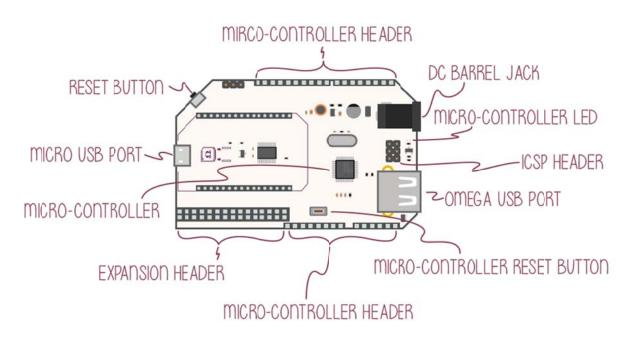
You can power the dock using a microUSB connection, or using the DC Barrel jack.
