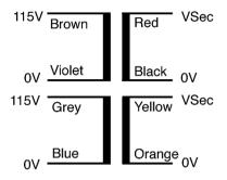
Primary 2x115V @ 50-60Hz Suitable for Series/Parallel connection
