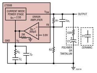
Figure 6. Model for Loop Response
