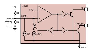
Figure 7. Undervoltage Lockout
