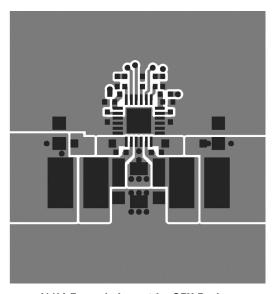
(11b) Example Layout for QFN Package
