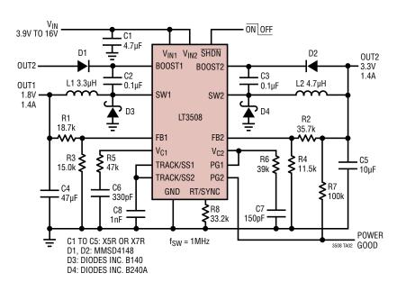
1MHz, 3.3V and 1.8V Outputs with Sequencing
