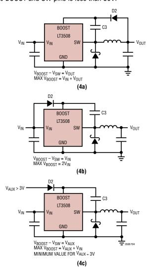
Figure 4. Generating the Boost Voltage
