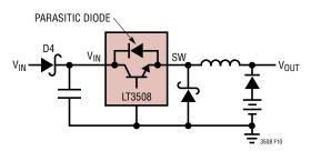
Figure 10. Diode D4 Prevents a Shorted Input from Discharging a Backup Battery Tied to the Output
