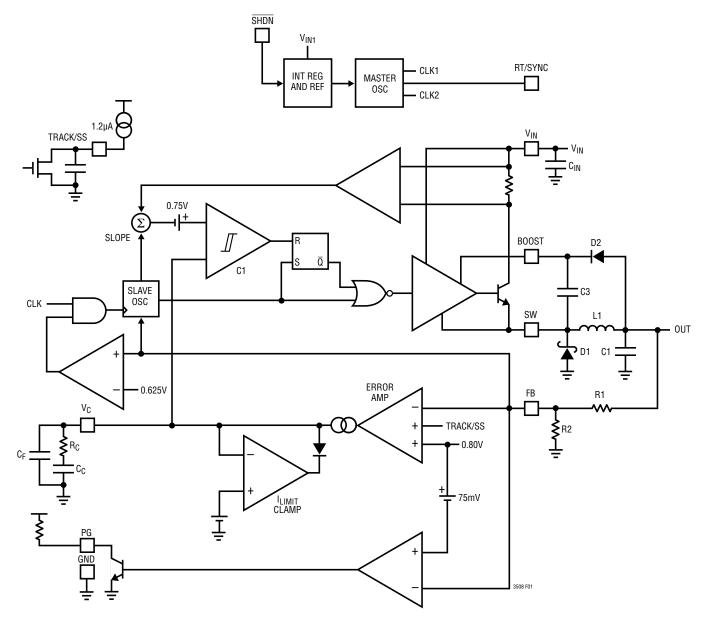
Figure 1. Block Diagram of the LT3508 with Associated External Components (One of Two Switching Regulators Shown)
