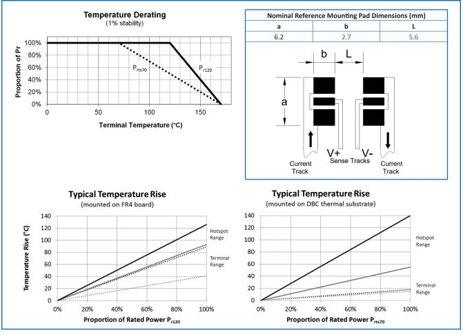
FR4 board details: 102x51mm, high T<sub>g</sub> FR4 board with 70 $\mu$ m (2 ounce) inner and outer Cu planes or similar substrate, such that terminal temperature is maintained at  $\leq$ 120°C.
