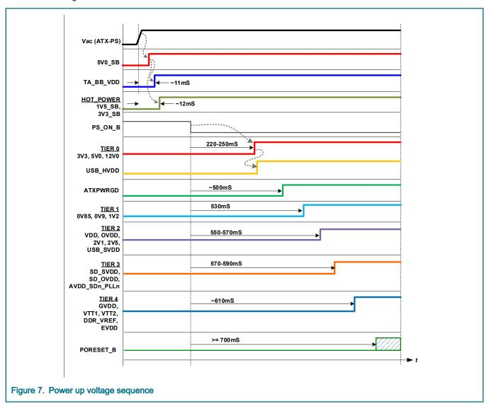
The LX2160ARDB follows the power supply sequencing requirements as detailed in QorlQ LX2160A Data Sheet.
