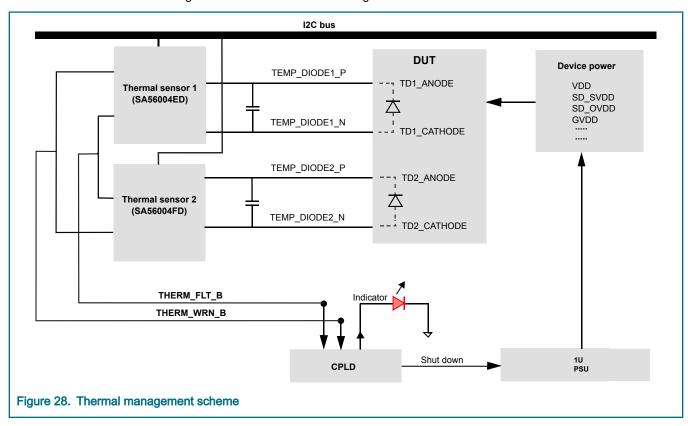
Thermal monitoring happens with no programming involved. However, if the thermal limit, by default set as 85 °C, is higher than desired, it will need to be re-programmed. To change the thermal trip point, issue the I2C writes listed in the table below.
