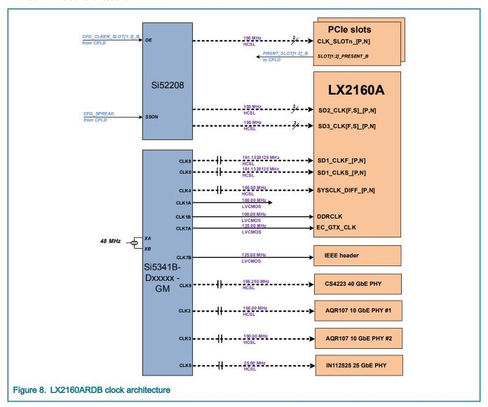
All the clocks are fixed frequency, and most are produced by the Si5341B or Si52208. The following table summarizes the specifications of each clock and the component that provides it.
