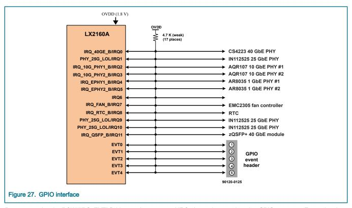
By programming the RCW "IRQ\_EXT" field properly, an unused IRQ pin can be reassigned to GPIO purposes. Event signals from EVT pins EVT[0:4] flow through a 5-pin GPIO header.
