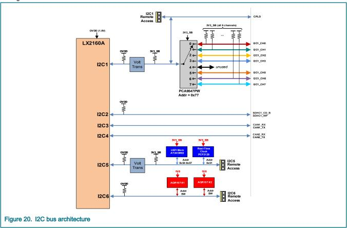
The multiplexer used for the I2C1 bus partitions the bus into eight sub-buses, called "channels." Software must program the multiplexer to access one of the eight I2C1 channels. All boot-software-dependent devices are placed on channel 0, or "I2C1\_CH0" as it is named. Channel 0 is the default selection upon reset so that software has immediate access to critical resources.
