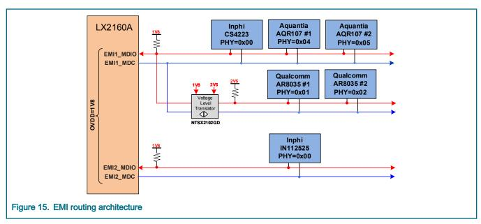
Both EMI1 and EMI2 operate at OVDD (1.8 V) levels. For devices not operating at 1.8 V, EMI signals are bi-directionally shifted to the compatible voltage using voltage level translators.
