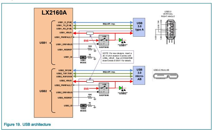
The USBx\_DRVVBUS and USBx\_PWRFAULT pins of each USB controller are connected to a programmable-current USB switch, NX5P3090UK (from NXP), for individual port management. The USB switch is powered from +5 V USB power supply. The USB1\_DRVVBUS/USB2\_DRVVBUS signal controls the VBUS drive for USB1/USB2 port. The USB1\_PWRFAULT/ USB2\_PWRFAULT signal gets power fault indications through the USB switch. The maximum allowed current consumption of a USB connected device is 2 A per channel.
