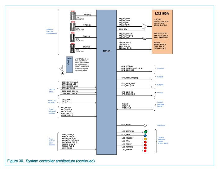
The system controller is implemented in a 256-ball micro-BGA Altera CPLD, EPM2210F256C5N.
