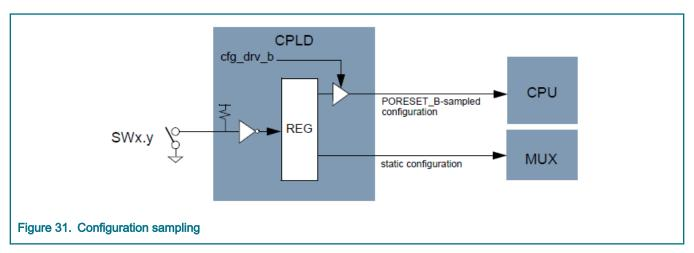
Note that switches cause a short to ground when closed. To make it easier to set and read switches, values are inverted in the CPLD, so that when a switch is on, the value used is 1.
